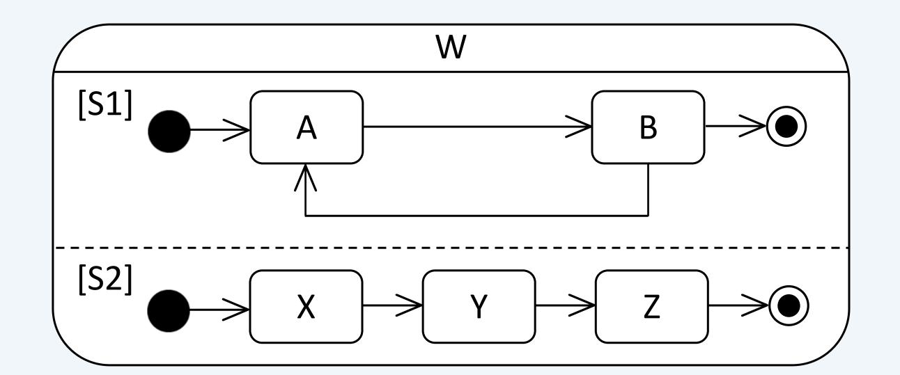
At any given time, one substate of each of the two orthogonal (=parallel) regions of **w** is active!
