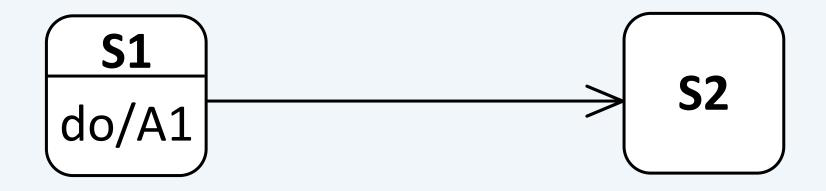
As soon as A1 is completed, a completion event is generated that triggers the transition to S2
