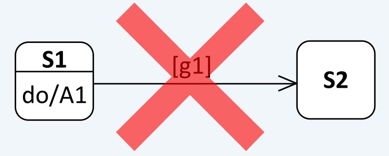
As soon as **A1** is completed, a completion event is generated and **g1** is evaluated. If **g1** is true, the transition to **S2** occurs. If **g1** is false, the transition can never take place
